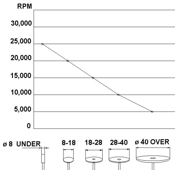
Please, keep the RPM according to below diagram against the accident.
